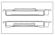
The broiler pan grid can be turned over to give two cooking positions.
